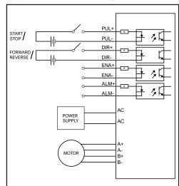
\*The typical connection of the drive switching to IO Mode
